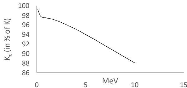
Fig. 3. Collisional Kerma,  $K_c$  against Energy.
